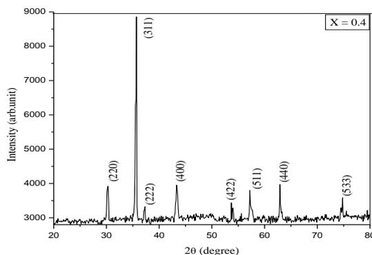
**Fig. 1: XRD patterns of  $Ni_{1-x}Cu_xFe_2O_4$  for  $x = 0.4$**
