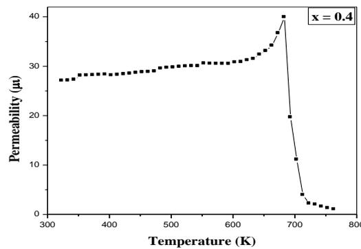
Figure 3: Permeability versus Temperature plot of  $Ni_{1-x}Cu_xFe_2O_4$  system at  $x = 0.4$
