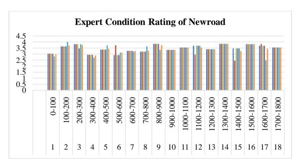
Experts view and suggestion on road condition rating based on site photographs were collected for different sections of road. The ratings of the sections were arranged to find out the most severe road section. The study shows that section 1400-1500 is the most severe on PrithiviChowk – Mahendrapool road section. Similarly, 1300-1400 and 1700-1800 sections were found to be the most severe on Zero Km – Hallanchowk road section.
